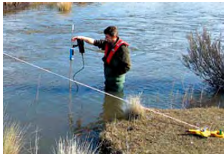
Above: Photo showing technician measuring the flow velocity and the water depth.
