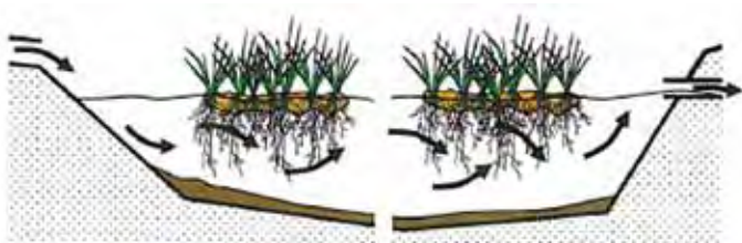
Above: Cross section of a typical floating treatment wetland system with partial cover of pond surface with floating wetlands. Figure courtesy of Heady & Tanner (2006)
